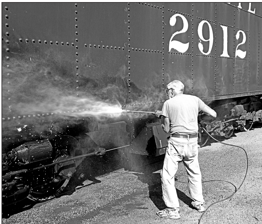
Karl Rethwisch power washing the 2912 tender on June 3, 2017, to prepare for painting. – Photo © 2017 Paul Brown.
